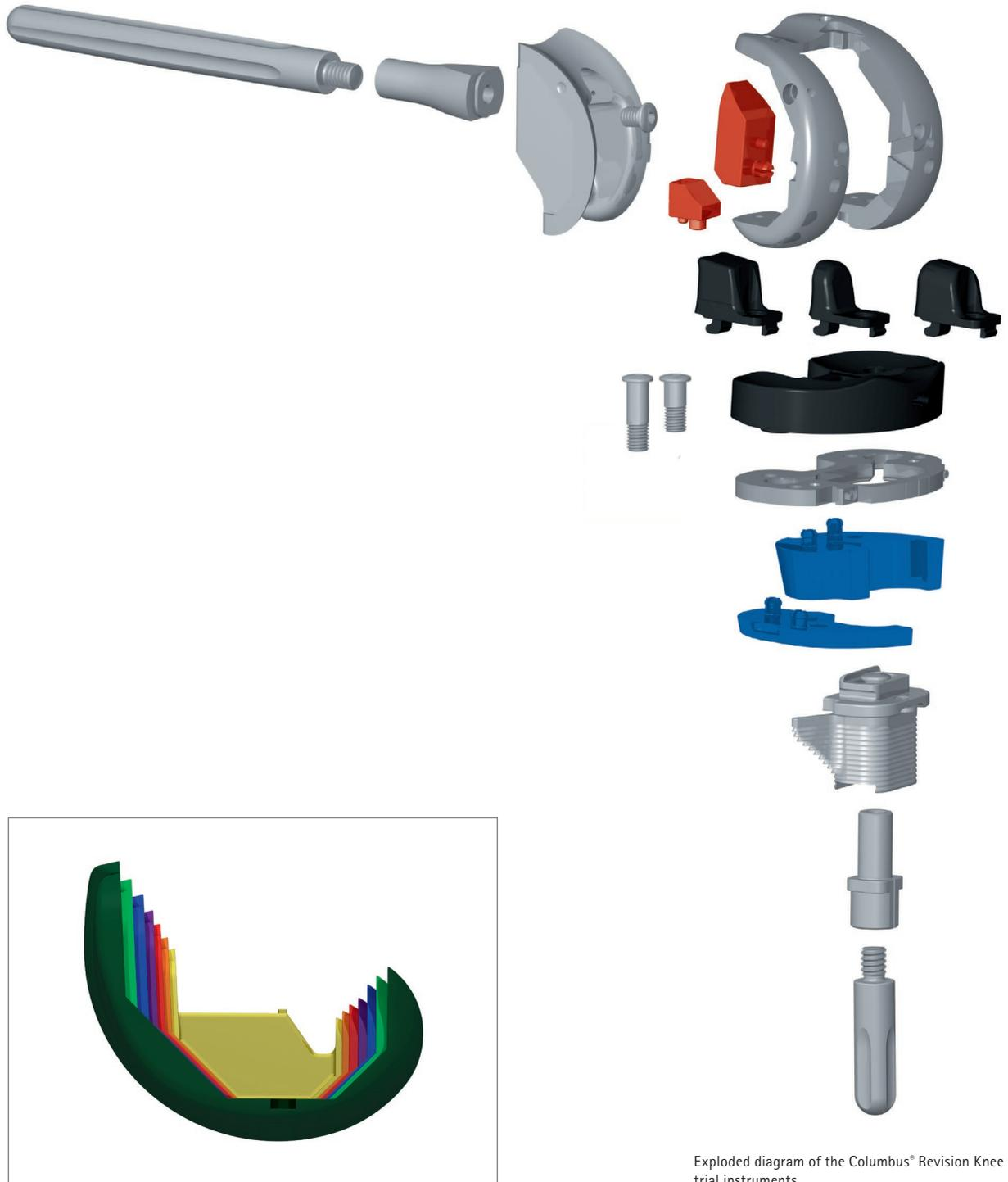
Exploded diagram of the Columbus® Revision Knee System trial instruments
