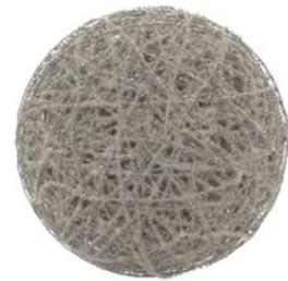
Cellulose fiber containing silver nanoparticles
